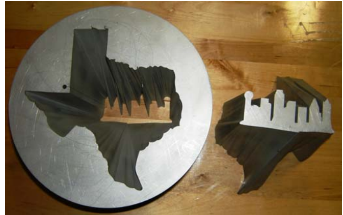
8"dia. Steel block with State of Texas on one side and skyline of Dallas on the opposite side -- All done with one cut!
